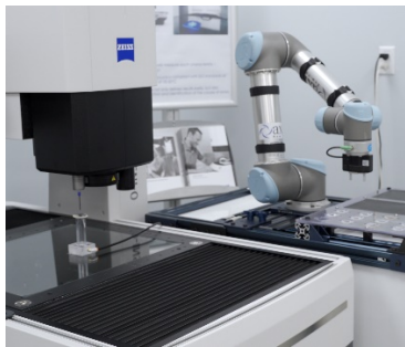
A Q-Span System with one gripper/caliper on a UR3e cobot enables "smart" machine tending of a CMM. The gripper/caliper makes preliminary measurements of parts before placing them in the machine.
