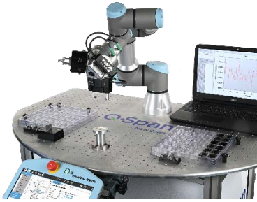
A Q-Span Workstation incorporates gripper/caliper, tool mounting, and software innovations in a robotic solution specific to QC measurement of small parts.
