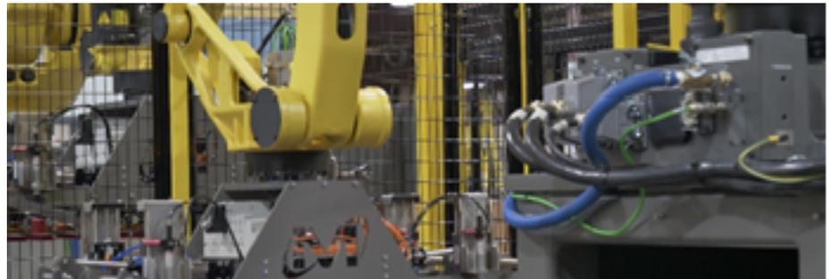
The robot picks up the cartons from a plastic belt conveyor from where the cases filled with sweet tea or juice arrive to be palletized.
