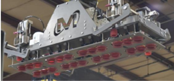
Cold resistant B75.20 silicone cups and SX12 vacuum pumps from Piab enable flawless gripping processes.
