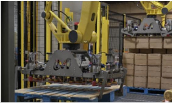
The system starts by picking up a pallet and placing it onto a roller conveyor with four mechanical clamps.
