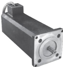
Based on our 230 VAC B and M Series, the Kollmorgen EB Series provides a high-performance explosion-proof servo motor suitable for applications where flammable vapors or gases create a potentially hazardous environment. These motors have been tested and proven capable of withstanding an internal explosion without bursting or allowing ignition to reach outside the motor frame.
