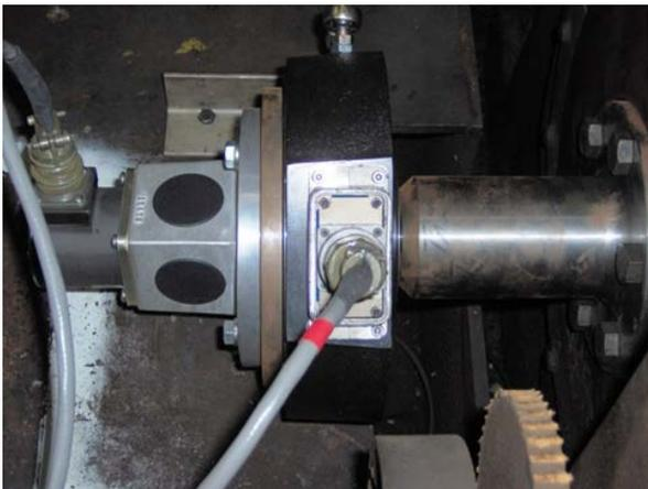
**Figure 1: Designed to operate without vulnerable electronics, resolvers like this R25 housed resolver (left) provide high-resolution, robust feedback solutions in demanding environments like steel mills.**
