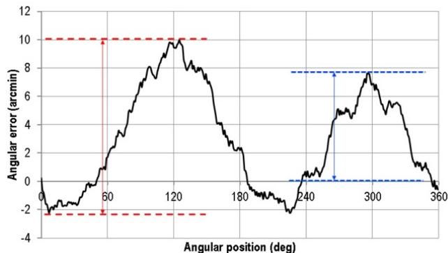
**Figure 2: Plot of error as a function of angular position over a full rotation shows peak-to-peak error (red) of 12 arcmin and +/- error (blue) of 8 arcmin.**
