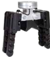
Parallel Hub Models Utilizes 2 finger arrays, with up to 5 fingers per array
