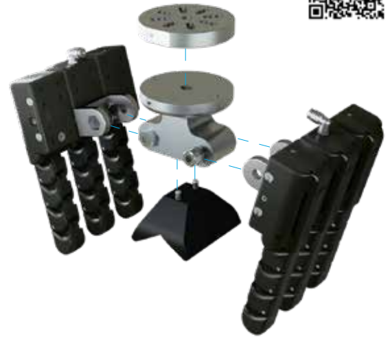
Parallel Hub Models Utilizes 2 finger arrays, with up to 5 fingers per array
