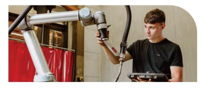
Cobots are lightweight, collaborative robotic arms designed to work safely alongside people to perform tasks that may be too dangerous, tedious, or strenuous for them to accomplish on their own. With advanced safety features, cobots are much safer than traditional robots, where most applications require little-to-no guarding or other safety devices.
