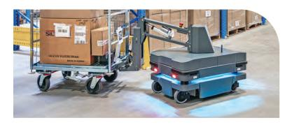
AMRs (Autonomous Mobile Robots) are designed to autonomate internal logistics processes by safely and independently navigating dynamically through busy work environments to complete tasks. Unlike AGVs (Autonomous Guided Vehicles), AMRs do not require a track or predefined paths, making path changes simple.
